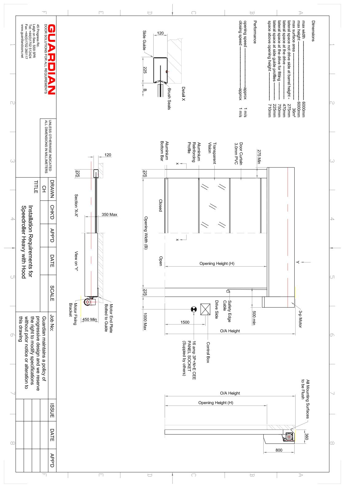
exclusion and climate control Functionality includes; energy saving, draught rolling door with electric drive. Applications are in industry and public utilities with exterior openings The Guardian Speed Heavy OUTDOOR is a rapid
