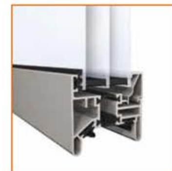
Panorama door 60 mm Triple Plexiglas Optical 40 mm (4-14.75-2.5-14.75-4 mm)
