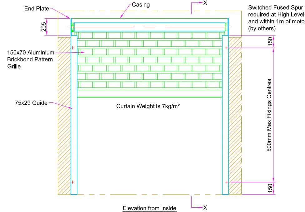
Switched Fused Spur required at High Level and within 1m of motor.
